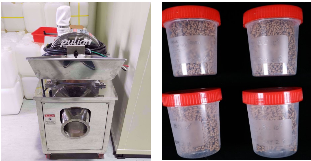
Fig. 3. Samples of microbial agents granules (right) from fluidized bed granulator (left).
